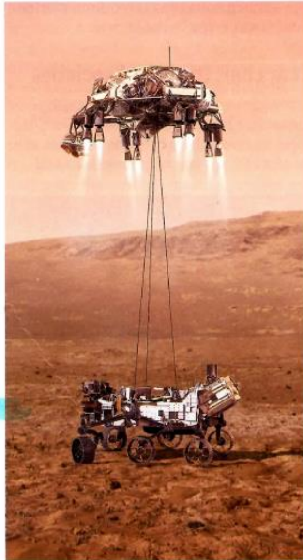
A "sky crane" landing device is designed to lower a 1-ton NASA rover to a soft landing on Mars.
